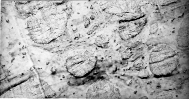
Figure 9: TEM micrograph of the PP/recycled-HDPE blend. Scale bar: 2.8\mu\text{m} . ( ——— ).
